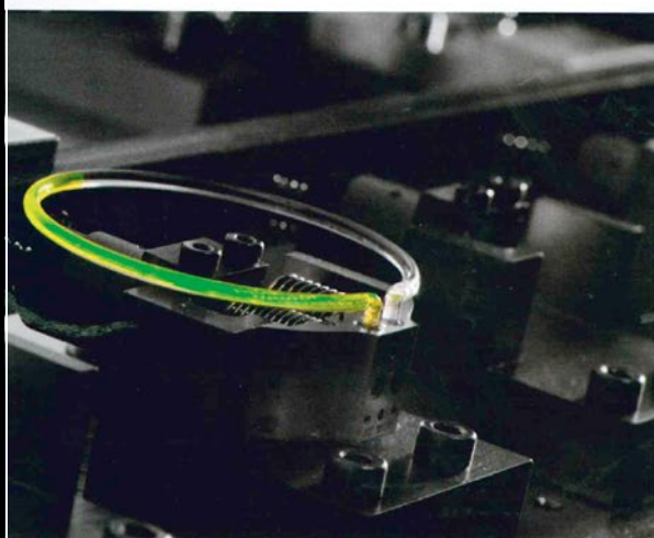
The H1 Azo Project by HYT works as a hybrid mechanical/fluid system - a watch movement activates pistons that display the passage of time by pushing a special liquid inside a graduated glass tube
